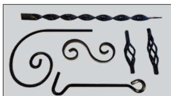
Examples of scrolls and twists possible with the Scroll Bender or Picket & Basket Twister Attachment.
